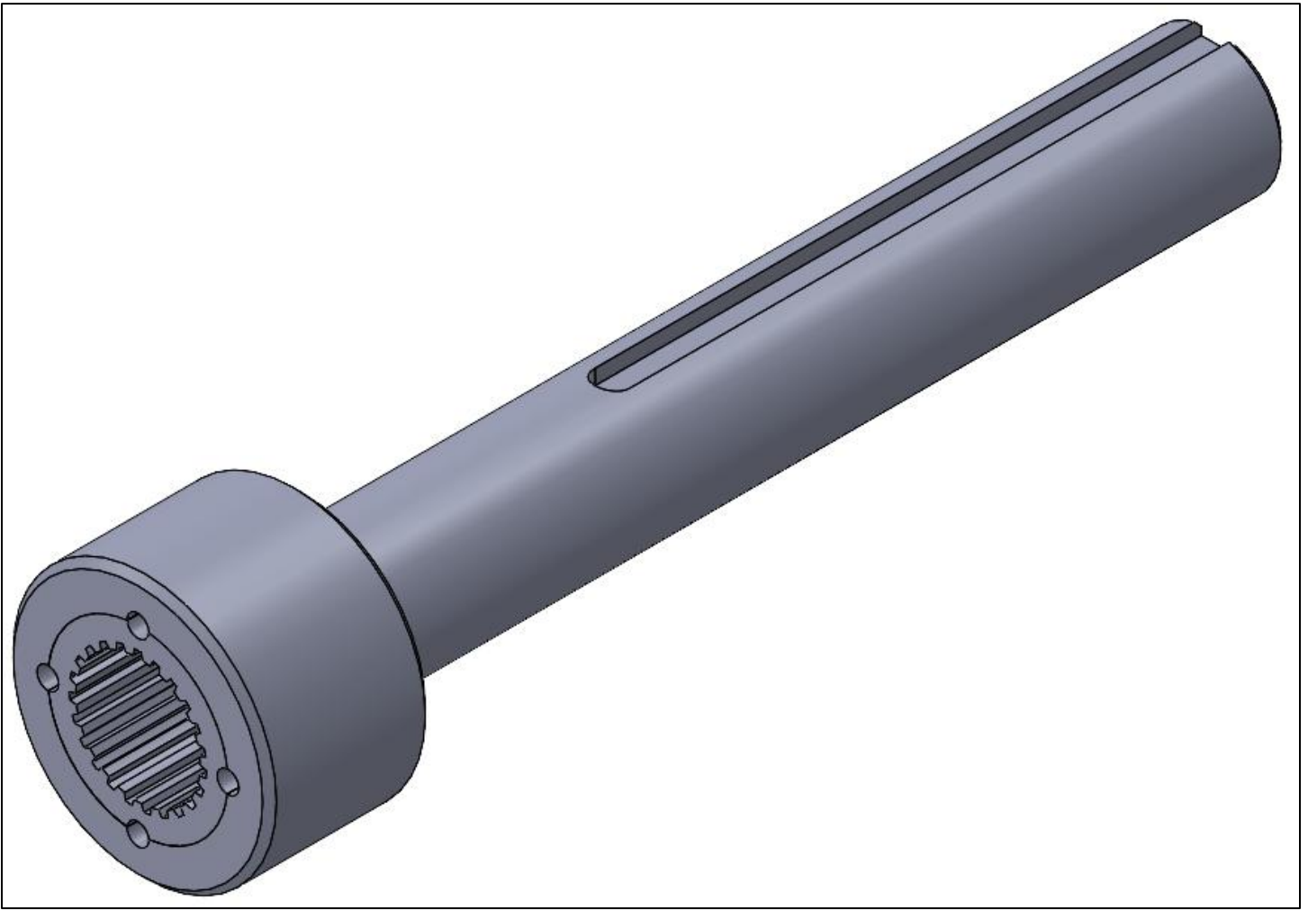
Figure 115: Output shaft with press fit internal spline and roll pin holes between the output shaft and spline pattern.
