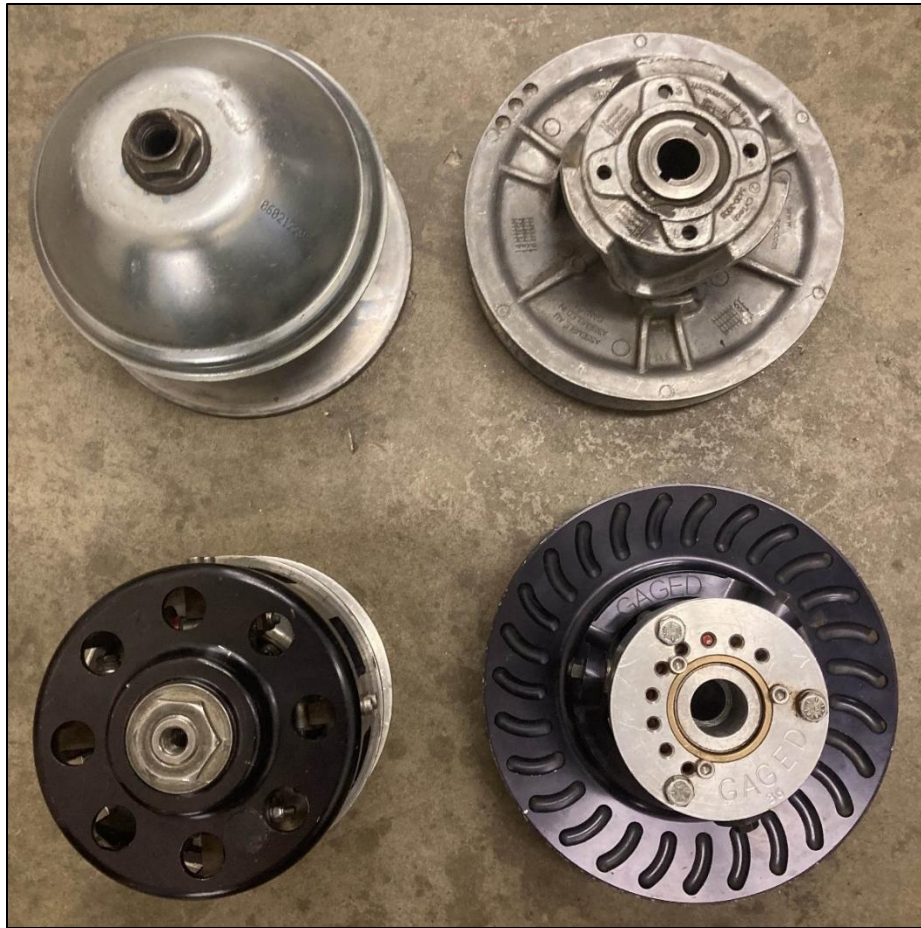
Figure 106 – Top: CVTech CVT; Bottom: Gaged CVT
